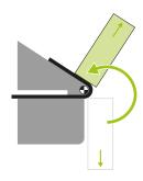
With adjustable bending centre the folding beam follows the radius beam perfectly.
