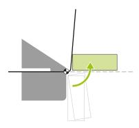
With fixed bending centre, thin material and adjusted folding beam. Good flexibility for angles and limited stress on machine and material.
