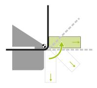
With adjustable bending centre the folding beam follows the material and bends angles correctly with even radius independent of the material thickness.
