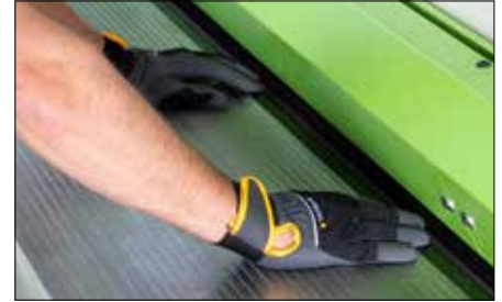
Hold down beam only 32 mm (1.25") from the cutting line for minimal waste.
