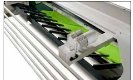
Sheet support in lower position for delivery of cut-off material to the front, operation controlled from CutLink.
