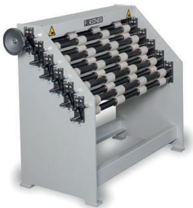
The guide rollers are movable in height, lifts up the sheet and create distance so that you avoid scratches in the lacquer layer.
