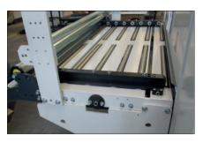
Optional: The coil guide is an important component for the function and accuracy of every system. The table has a fixed and a manually adjustable coil guide with ball bearings. The adjustment of the movable coil guide is done by a hand wheel. This specific table has rollers integrated in the table to ensure a smooth surface. The table with roller guide is available in both 1250 and 1500 mm.
