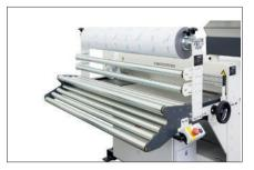
Optional: The film applicator can basically be mounted on any table. Using the deflection rollers and the fully rubberized feed rollers, the protective film is pressed on almost bubble and wrinkle-free. The decive type F-AG z2mo has an additional arm with tension spring for tensioning the film during the return movement. This design is only applicable for single decoiling systems. The film applicator is available in both 1250 and 1500 mm.
