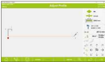
Draw your own profile and set the measurements, angles and values for radial bending.
