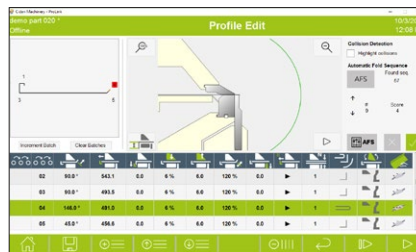
This function automatically calculates bending sequence, analyses possible collisions and provides information in graphic display for the operator.
