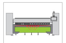
**Crowning of the folding beam** rail gives perfect right angles and measurements along the entire profile. On Z-machines this function is controlled from the values programmed and adjustment is completely automatic.
