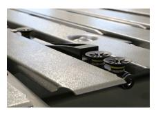
With **vacuum grippers** in the backgauge you can fold details with less assistance from the operator and with greater precision. This also shortens cycle times.
