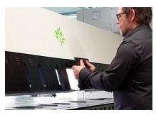
In **tool change position**, changes are made quickly and safely. The control system confirms that the right tool has been chosen and is correctly mounted.
