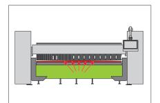
**Crowning of the folding beam** rail gives perfect right angles and measurements along the entire profile. On Z-machines this function is controlled from the values programmed and adjustment is completely automatic.
