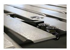
With **vacuum grippers** in the backgauge you can fold details with less assistance from the operator and with greater precision. This also shortens cycle times.
