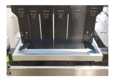
**Collapsable Corner Tools** (optional). With Collapsable corner tools, removing parts with inward flanges from the machine is simple.
