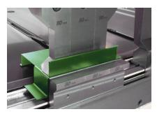
**Multifold** is standard for all Z-machines, i.e. all tooling is divided. Combined with height adjustable back gauge, Multifold gives unsurpassed flexibility for profile geometry.
