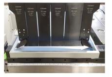
**Collapsable Corner Tools** (optional). With Collapsable corner tools, removing parts with inward flanges from the machine is simple.
