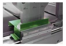
**Multifold** is standard for all Z-machines, i.e. all tooling is divided. Combined with height adjustable back gauge, Multifold gives unsurpassed flexibility for profile geometry.
