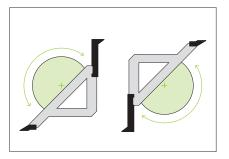
With the **combi beam** you have the advantage of a straight rail with angled upper beam and high divided tooling with the same tool set-up and changes can be made in less than ten seconds.
