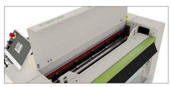
To simplify the adjustment of the slitting blades, we have installed a LED slitting blade illumination. This gives the system a visual highlight and contributes to the safe and quick adjustment of the slitting blades.
