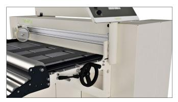
The adjustment of the table guide is now located on both sides of the table in the new SLIT series. The handwheel can be mounted on both sides, as the locking of the guide now takes place via a new concept. Furthermore, the spindle for guide adjustment has been optimized, you can now achieve twice the length of the movement with one rotation, which will make your sheet metal change even more efficient.
