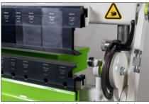
Corner tools as standard for maximum flexibility. Tool height in lower beam is 60 mm and the tools in the folding beam are 94 mm.
