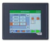
With CutLink set to Automatic mode, you can program 10 lines with different dimensions and quantities to be processed in sequence. You can save the settings in the system memory.
