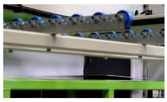
When the sheet support is pulled back, the sheets fall straight down for soft landing on the material wagon (option), with no risk of damage.
