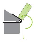
With adjustable bending centre the folding beam follows the radius beam perfectly.
