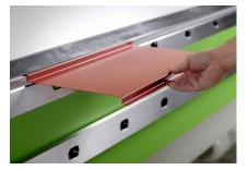
**Master of fine detail.** With the CIDAN concept of spring steel gauging fingers and the narrowest folding rail on the market, you get precision, finish and flexibility, even for very fine gauge measurements, down to 3 mm.
