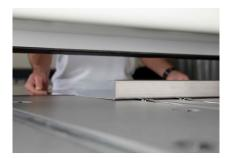
**Generous and ergonomic.** The opening height is 150 mm. Perfect for fast, efficient and ergonomic profile handling.
