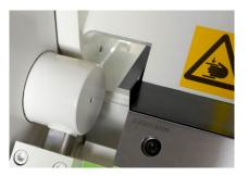
**Spacious recesses** in the clamping beam. 49 mm high and 57 wide, the recesses allow greater flexibility and make complex folding much easier. With the new F and FS/FX you have new possibilities and can achieve the results you want both faster and trouble-free.
