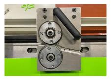
With a simple **rotary shear** attachment along the bend line, you can easily cut off blanks or folded profiles. (Only F41.)
