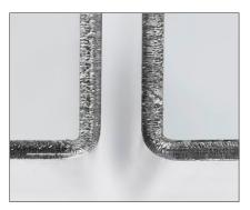
The radius differences are clearly seen in the illustrations above. With a fixed bending centre (left) the radius is uneven and the material is unevenly distributed. With an adjustable bending centre (right) the radius is even and there is less stress on the material.
