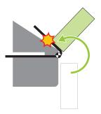
With fixed bending centre there is considerable angle error and a clear risk that the folding beam rail and radius rail "collide" leading to a great deal of wear on the machine or breakdown.
