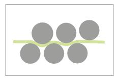
The STRAIGHT machine has 6 automated straightening rollers to remove coil set and give customers flat material every time.
