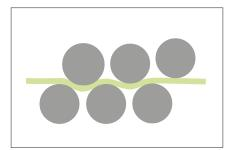
The STRAIGHT machine has 6 automated straightening rollers to remove coil set and give customers flat material every time.
