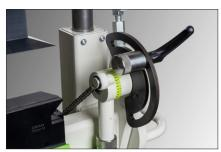
Easy setting of folding angles with bending angle stop.
