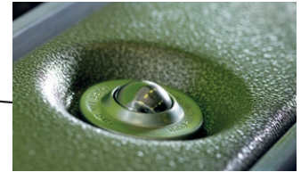
Ball casters in the back gauge system protect the material and facilitate rotating the material. Alternatively you can choose brushes for the back gauge table.
